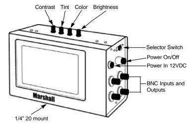
when power is supplied to the monitor. The monitor also has a 1/4-20 mount located on the bottom of the unit. This is useful when mounting the monitor on the top of a camera by using a hot shoe mount (Marshall part# V-LCD-MT) or other mounting devices.
